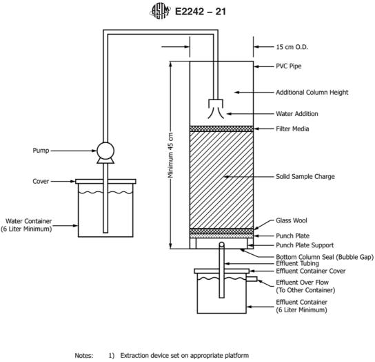
above effluent container to allow gravity flow of effluent and drain.
